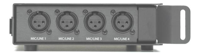
There are four balanced XLR **MIC/LINE** inputs on the left side (input side) of the mixer. (Although earlier units were labeled as **Mic 1** thru **Mic 4**, in actuality these inputs are switchable for either MIC LEVEL or LINE LEVEL inputs. The term "Mic" was used informally to differentiate inputs from outputs.)
