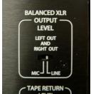
bottom of the mixer to select MIC LEVEL output for the main XLR's.
