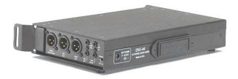
The On/Off switch is located on the right side (output side) of the mixer, towards the back. When you power up, the red LEDs on the face of the unit will indicate battery or external power source. You can operate the ENG 44 from AC by plugging in the 12v power adapter that comes with the unit.
